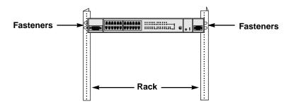
Figure 2-4 Rack-mounting the FN10
